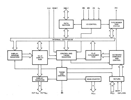
The command is then decoded and the appropriate function is set. The timing control contains the basic timing counter chain. The first counter is a  $\div$  N prescaler that can be programmed to yield an internal frequency of 100 kHz which gives a 5.1 ms keyboard scan time and a 10.3 ms debounce time. The other counters divide down the basic internal frequency to provide the proper key scan, row scan, keyboard matrix scan, and display scan times.
